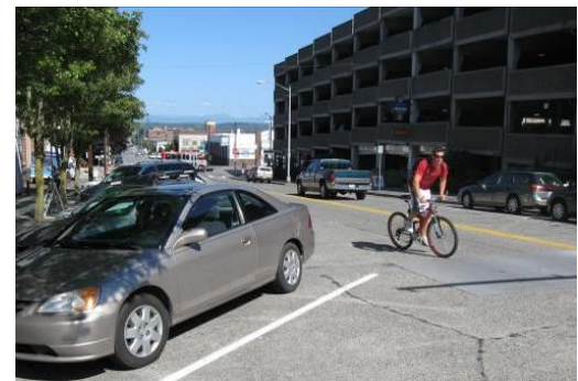
Changing angle parking to parallel parking will provide room for bike lanes on California Street.
